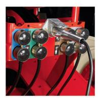
The HydraFlow® Closed Center Load Sensing Hydraulic System provides required pressure for efficient operation of implements. When not loaded, the system operates in low pressure power-saving mode, creating a reserve for the transfer of all power.
