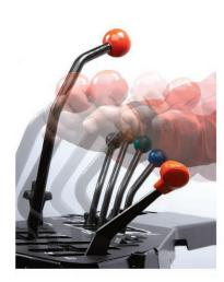
Quadshift® III 12x4 manual transmission is standard equipment. The transmission has 3 speed ranges.
