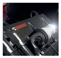
RSM 2375 tractors are equipped with 10.8L QSM 11 engines. Powerful, efficient, adapted to operate in the non-friendly environment, these engines are the result of decades of research and cutting-edge innovations. They will always start in any weather, generating virtually no smoke, unparalleled life, minimum noise at high speeds, and easy drive control
